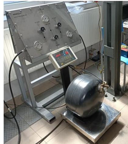
Fig. 3. Station for producing fuel blends
